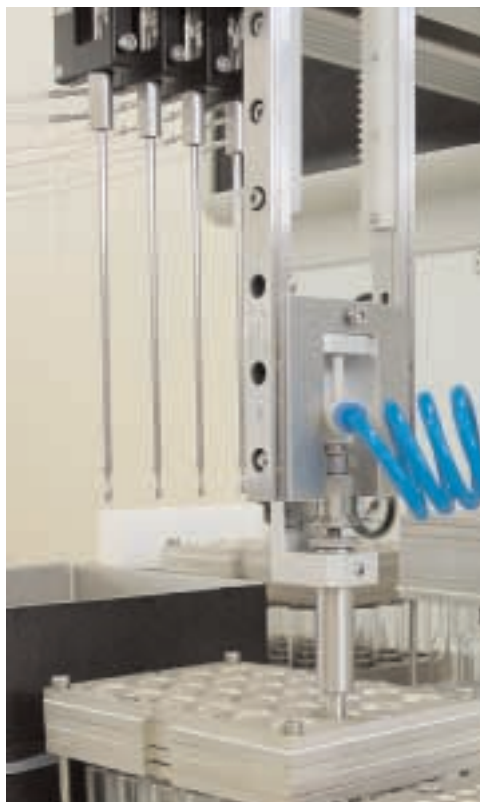
Figure 5: Pick-up Powder Tool for Distribution of Synthesis Resin and Scavenger Resin
